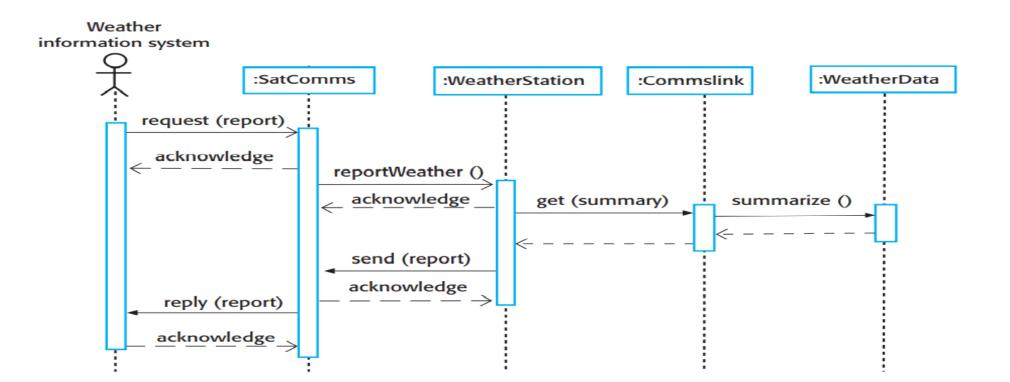
1. The **SatComms** object receives a request from the weather information system to collect a weather report from a weather station. It acknowledges receipt of this request. The stick arrowhead on the sent message indicates that the external system does not wait for a reply but can carry on with other processing.
