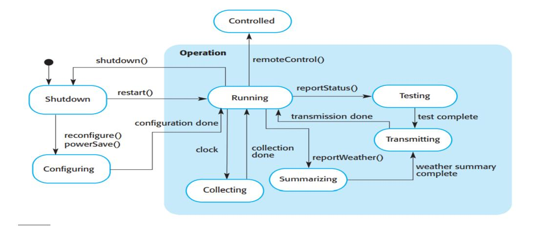
1. If the system state is Shutdown, then it can respond to a restart(), a reconfigure() or a powerSave() message. The unlabeled arrow with the black blob indicates that the Shutdown state is the initial state. A restart() message causes a transition to normal operation. Both the powerSave() and reconfigure() messages cause a transition to a state in which the system reconfigures itself. The state diagram shows that reconfiguration is allowed only if the system has been shut down.
